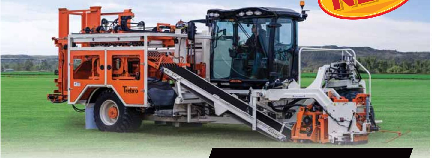
Fully Self-Contained AUTOMATIC SLAB HARVESTER
