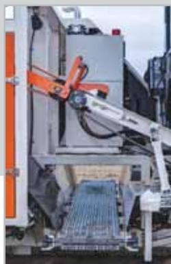
Cross-conveyor scrap dump - puts scrap out of the way
